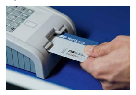
Part of the Follow- Print- Solution: the value card accounting system, which is also used for the identification of the user print jobs.
